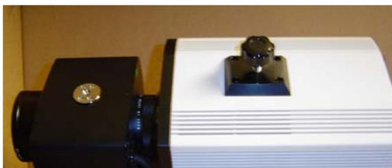
**ChemiDoc XRS camera with thumb screw**
