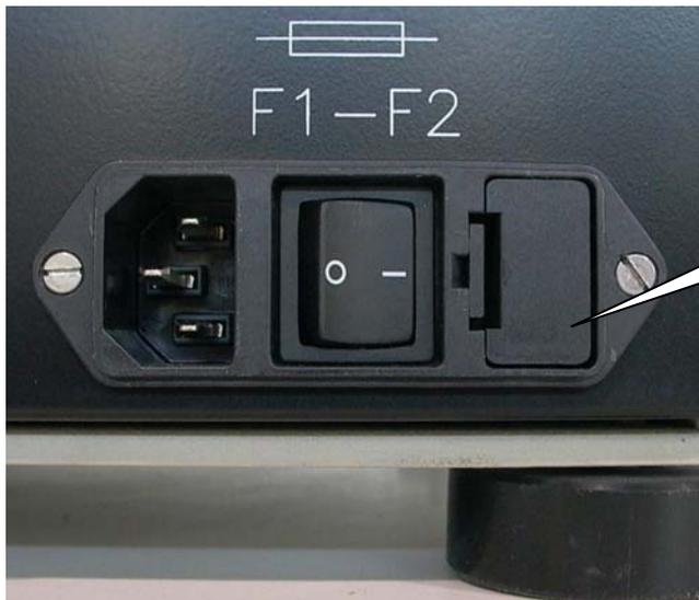
Fuse F1 and F2 are located in this drawer. Use a screwdriver and pull the drawer out to see the fuses.
